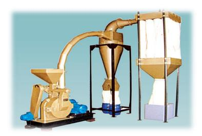
♣ Standard installation is with mill having in-built classifier gap plate, fan, cyclone collector and fabric type dust collector with suitable stands. At the outlet of cyclone, y-piece or/and rotary airlock valve is provided depending upon the application and fineness of end product. For sticky and large size installation additional suction blower is recommended.
